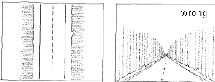
Figure 8.6 Density of the field of view is low; monotonous and long straight-ahead section stimulate subconscious speeding up (Birth, et. al 2004)
